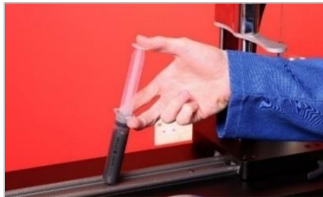
FIGURE 24 - Application de graisse
