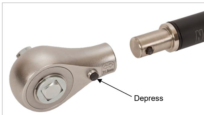
**NOTE: All NorTronic® tools are Torque Handles with a 16 mm spigot. Should you wish to change to a different spanner end fitting, depress the plunger on the ratchet head and pull to release.**
